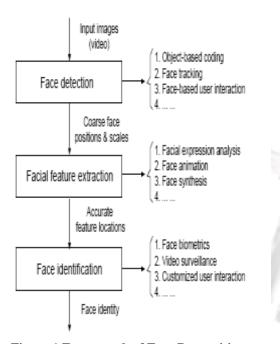
Figure 1.Framework of Face Recognition system
