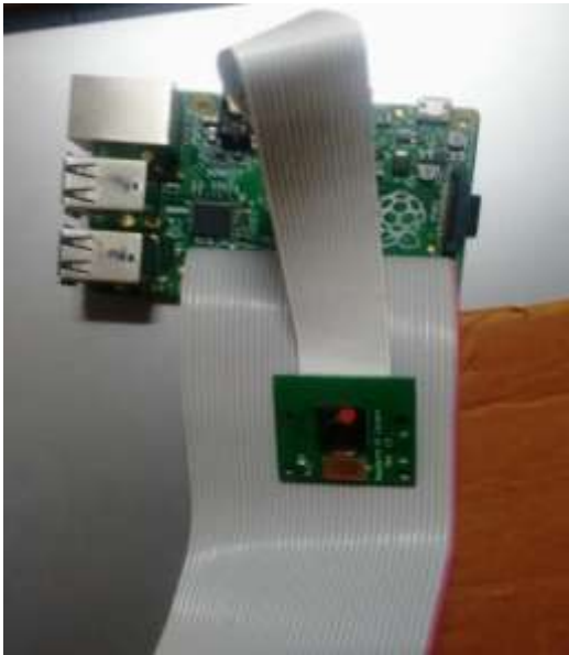
Fig. 5. Mid-sized Raspberry Pi connected to pi camera
