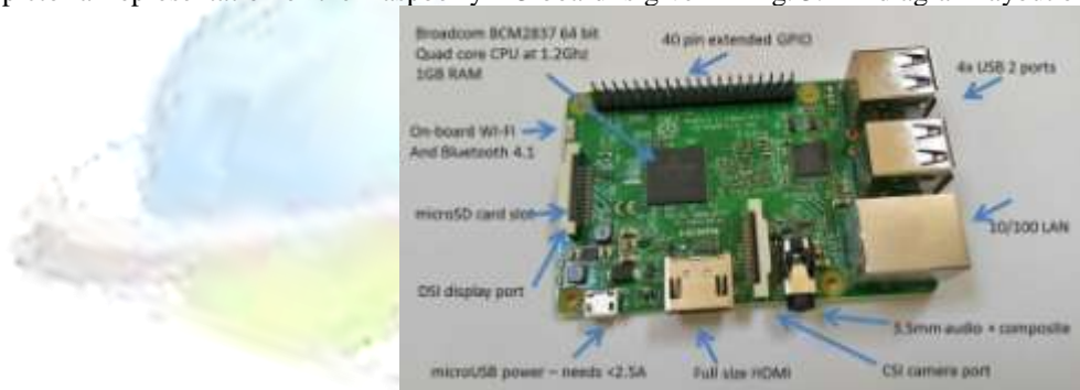
Fig. 3: Parts Of A Raspberry Pi 3 Board
