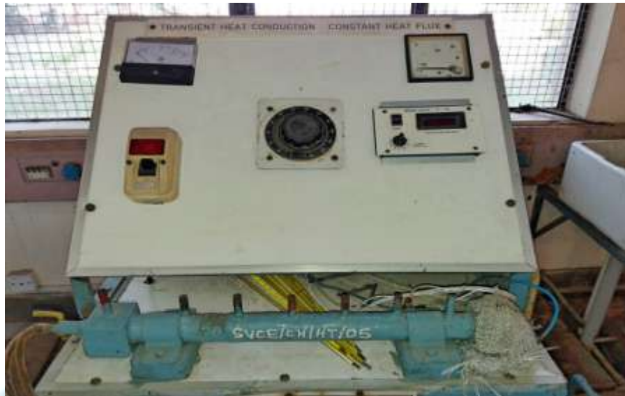
Fig. 1: Experimental setup for Transient Heat Conduction With Constant Heat Flux
