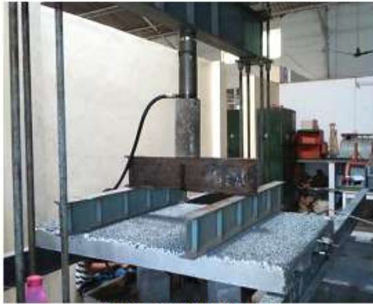
Figure 3 Slab testing setup
