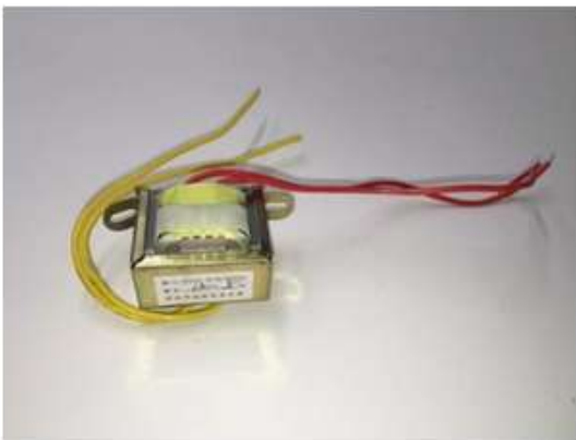
Fig.4: Potential transformer (12v)
