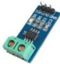
Fig.3: Current sensor ACS712
