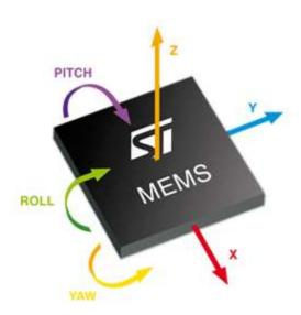
The MEMS Accelerometer usually comes in the smallest surface mount package and can detect acceleration in up to 3 axis. This tutorial will cover capturing data for onle one axis. The PIC will be used to capture the data and make sense of it.
