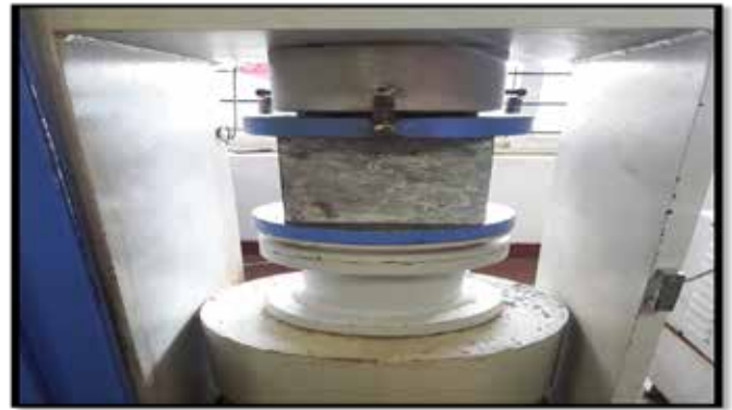
Fig 5 : Experimental Set up for Compression Test
