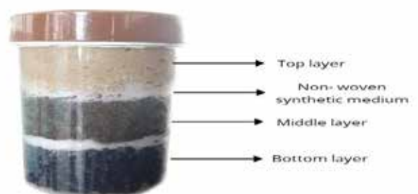
Fig 2 : Material Arrangement In Filter Bottle
