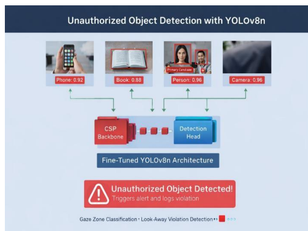
Fig 4: Unauthorized Object Detection Pipeline — yolov8n • Multi-Class Detection (Phone, Book, Person, Camera) • CSP Backbone • Real-Time Alert System
